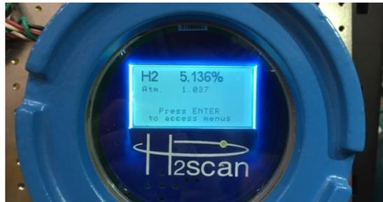
It has long been standard practice to use analyzers like thermal conductivity devices (TCD) or gas chromatographs (GC) to measure the hydrogen, but these suffer from known limitations compared to the accurate, real time, continuous measurements available from the H2scan solid state sensors.
